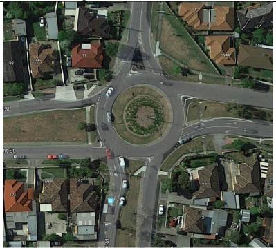
Large roundabout, difficult to cross, fast moving traffic with few gaps. The complexity of the intersection (number of movements to account for and multi-lane elements) adds to the difficulty.
