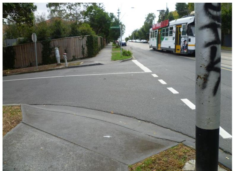
Figure 25 – poorly oriented kerb ramps, and corners that allow higher speed turning, Hawthorn Glen
