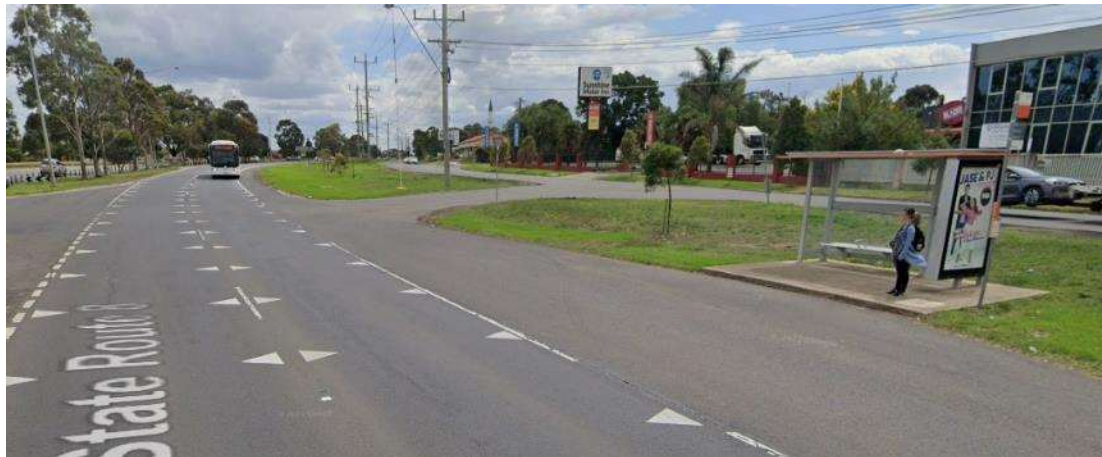
Figure 53 A person waits for bus on Ballarat Rd, Ardeer. Wire rope barriers in the median and guardrail on the opposite side of the road, in addition to the high speed and volume of traffic, make crossing directly to or from the bus stop extremely difficult and dangerous (Image source: Streetview, Google Maps, February 2020)
